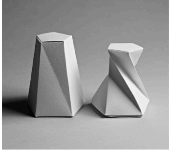
Figure 1: A bi-stable origami column by Paul Jackson [12]. (Left) The vertical valleys are unfolded and vertically extended. (Right) The top part is rotated clockwise and the height is lowered.
